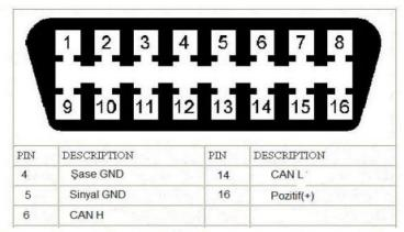
NOTE: In case the emulator does not work in this connection, the emulator GND cable must be connected to the 5.pin
