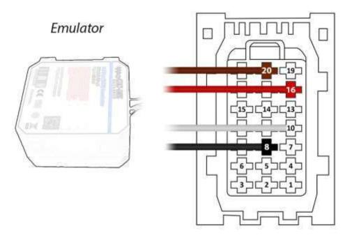
Brown (Emulator side) > Pin20 on socket side Red (Emulator side) > Pin16 on socket side White (Emulator side) > Pin10 on socket side Black (Emulator side) > Pin8 on socket side
