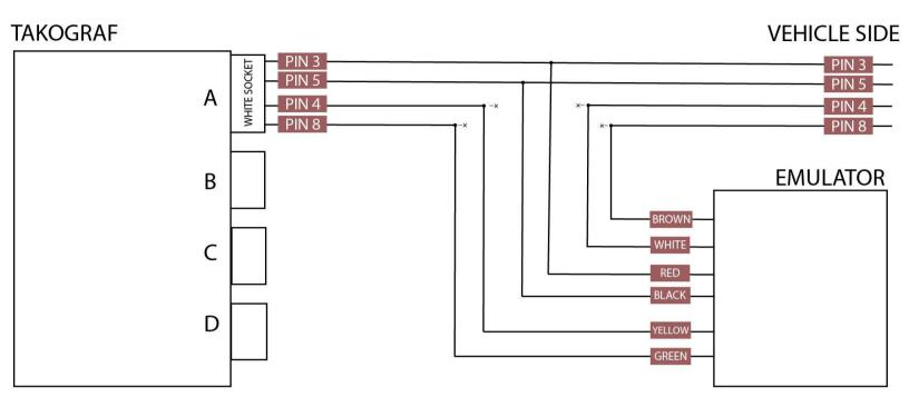
The ignition must be off during installation. Errors should be deleted after the installation.
