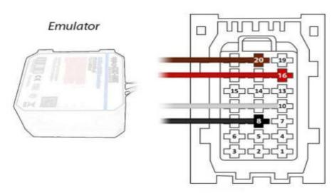
Brown (emulator side) > Pin20 on the socket side Red (emulator side) > Pin16 on the socket side White (emulator side) > Pin10 on the socket side Black (emulator side) > Pin8 on the socket side
