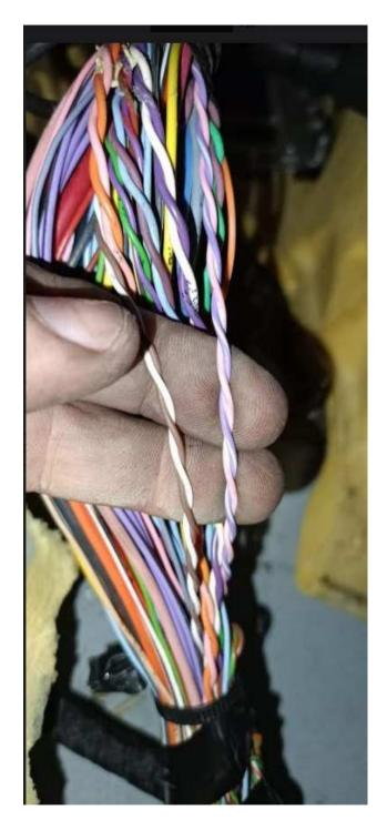
If the vehicle does not have a Black-White and Pink-White CAN line; The emulator Yellow cable should be connected to Purple-White, and the emulator Green cable should be connected to Pink-White.
