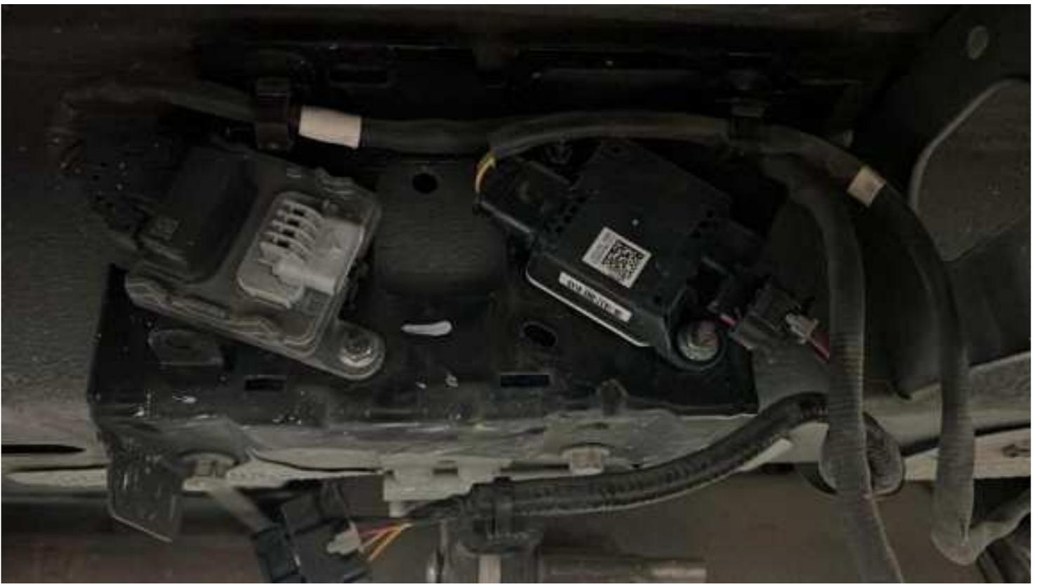
Pull out the PM sensor and downstream NOx sensor.
