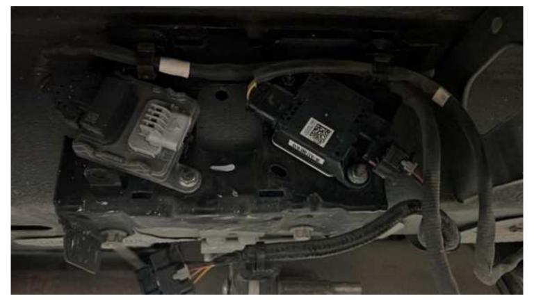
Pull out the PM sensor and downstream NOx sensor.
