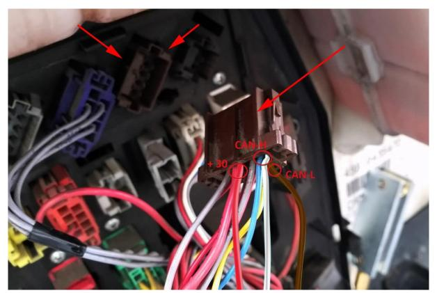
To connect AdBlue emulator we need to use these wires for CAN LOW, CAN HIGH and +30 connection (DAF LF EURO 4 / EURO 5 version).
