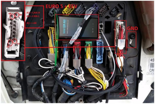
Connect AdBlue emulator CAN HIGH, CAN LOW and +30 wires to corresponding pins (DAF LF EURO 5 + EEV version).
