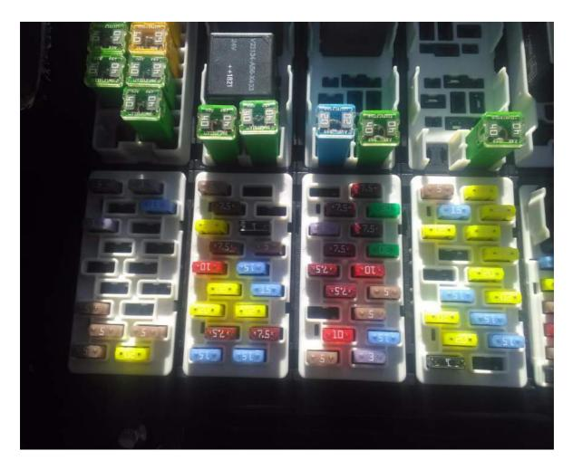
Firstly the vehicle must not be working. Then, as shown above, the fuse box is opening and the fuse that writes the Nox sensor in the vehicle booklet is take off.(It can be 33 or 36 numbered).
