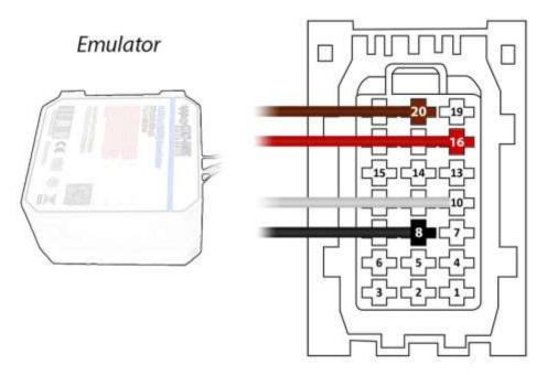
Brown (Emulator side) > Pin20 on the socket side Red (Emulator side) > Pin16 on the socket side White (Emulator side) > Pin10 on the socket side Black (Emulator side) > Pin8 on the socket side
