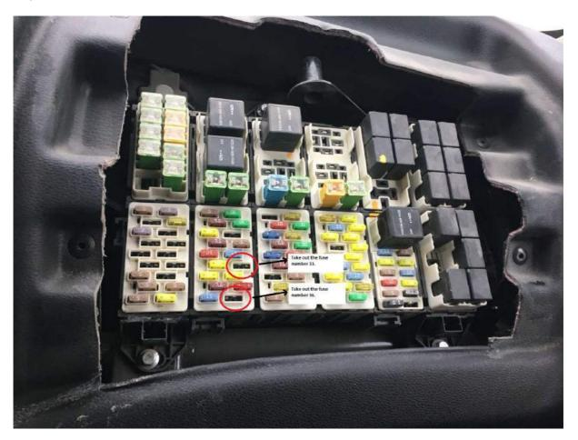
First of all, the vehicle must not be working. Then, as shown above, unscrew the fuse box 33 and the fuse 36 in the marked place.
