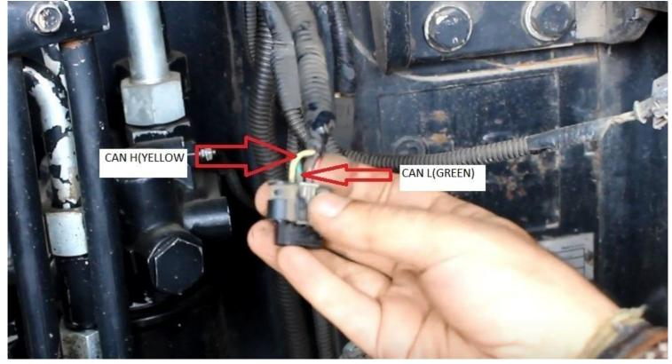
The brown and white wires in the emulator must be connected to the green and yellow wires extended from the nox socket. The following image shows the connection details.
