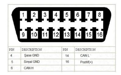
NOTE: If the Emulator does not work in this connection, the emulator must be connected to the GND cable to the 5th pin.
