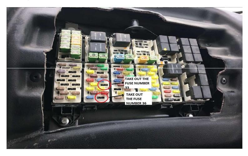
First of all the vehicle should not be working. Then open the fuse box as shown above and remove fuse 33 and fuse 36 at the marked location. Then the black cable (GND) of the Adblue emulator is connected to the 4th pin from the back of the -OBD socket, the red wire (positive +) - 16. pin, white wire (CAN H) - 6. Pin and brown cable (CAN L) -14. Connect the pine. You can then run the vehicle.
